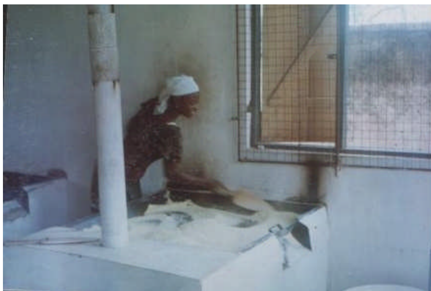
Figure 4. Gari frying in a sheltered communal fryer with chimney
