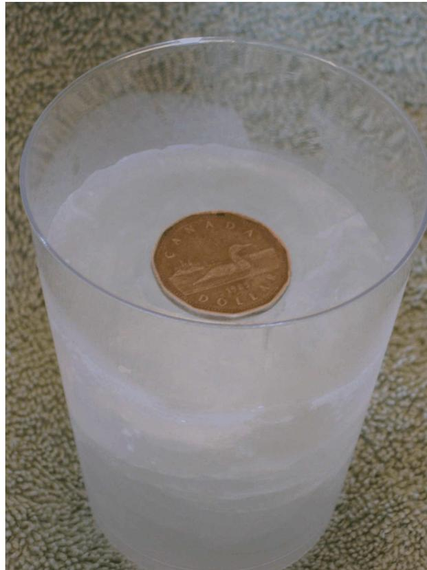
**A simple device for detecting thawing in your freezer**
