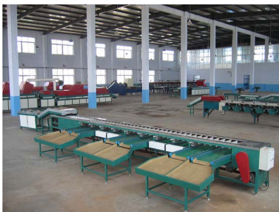
Figure 7: Machinery classification of apples
