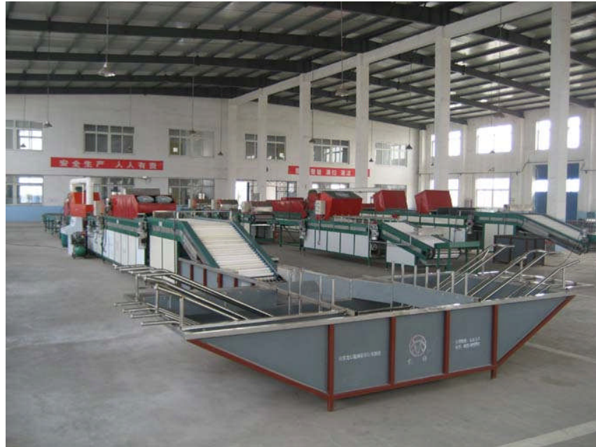
Figure 9: Equipment used for apple washing and waxing
