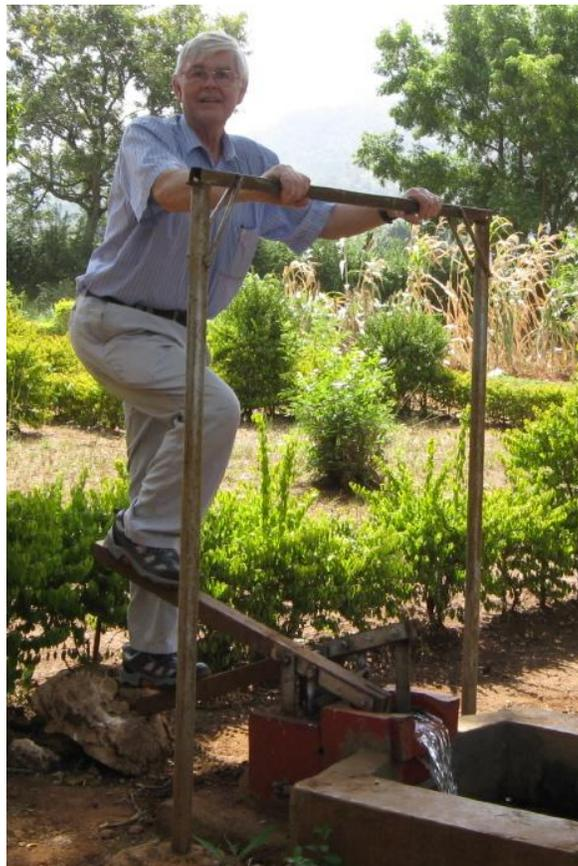
**Using a Concrete Pedal Pump**
